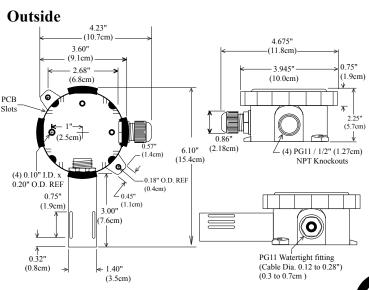
For CE compliance, sensor leads must be no longer than 3 meters in length. Additionally, certain product variations may not be CE compliant. Contact ACI for further details
