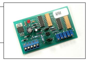
on input) on the ARM. The offset of the output can be adjusted anywhere from +/- .25 to +/- 20 VDC for the ARM
