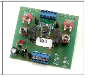
output and vary the analog signal independently. Each output can have a different span and be analog current or voltage. When a switch is in manual position, an alarm output contact is made or broken (optional) to indicate override is in effect.
