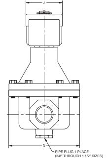
Must be mounted with solenoid upright or horizontal on 3/8" to 1 1/2" pipe sizes. For 2" to 3", must be mounted with solenoid vertical only.
