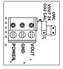
Fig. 6: J1 Set for 0 to 10 VDC Output
