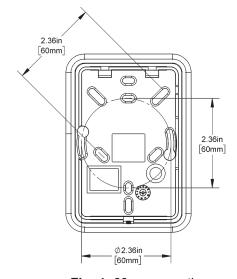
**Fig. 4:** 60mm mounting base dimensions
