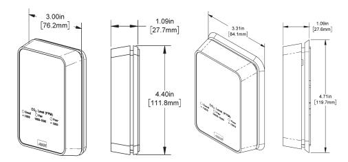
**Fig. 1:** BAPI-Stat "Quantum" CO<sub>2</sub> Sensor (standard mounting base at left and 60mm mounting base for European wall boxes with 60mm mounting centers at right)
