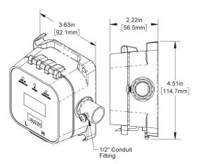
\*BAPI recommends that you do not run wiring for the pressure transmitter in the same conduit as line voltage wiring or with wiring used to supply highly inductive loads such as motors, generators and coils.
