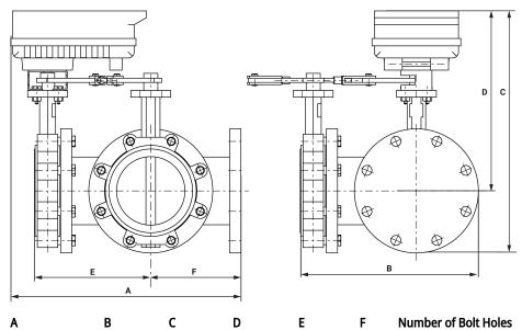
Valve with PR Actuator
