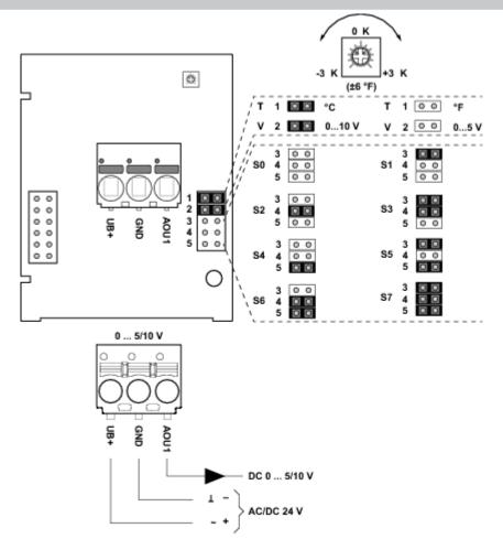
the adjustment of the measuring ranges is made by changing the bonding jumpers the output value in the new measuring range is available after 2 seconds
