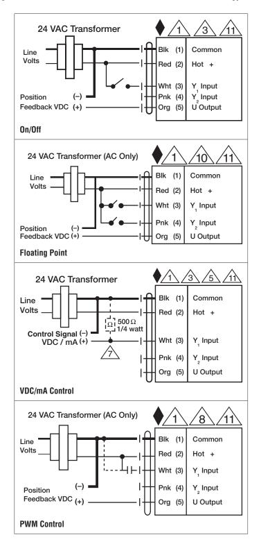
Modulating, Electronic Fail-Safe, Linear, 24 V, Multi-Function Technology®
