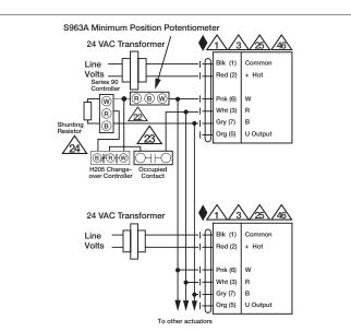
Multiple Actuators with Minimum Position Potentiometer
