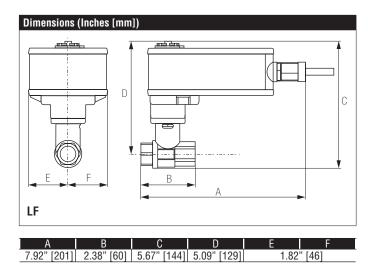
LF24-SR US, Valve Actuator Modulating, Spring Return, 24 VAC for 2 to 10 VDC or 4 to 20 mA Control Signal
