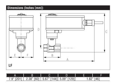
LF24-SR US, Valve Actuator Modulating, Spring Return, 24 VAC for 2 to 10 VDC or 4 to 20 mA Control Signal
