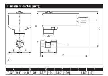
Modulating, Non-Spring Return, 24 V, for 2 to 10 VDC or 4 to 20 mA
