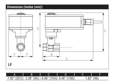
TR24-SR/300 US Modulating, Non-Spring Return, 24 V, for 2 to 10 VDC or 4 to 20 mA
