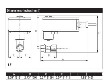
LF24-MFT-S US, Valve Actuator Modulating, Spring Return, 24 V, Multi-Function Technology®
