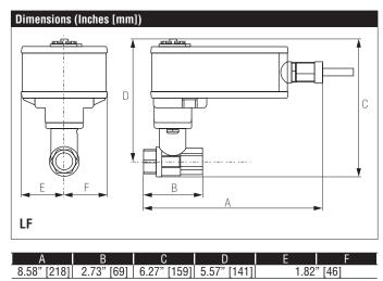
LF24-SR-S US, Valve Actuator Modulating, Spring Return, 24 VAC for 2 to 10 VDC or 4 to 20 mA Control Signal
