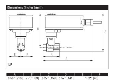
LF24-SR-S US, Valve Actuator Modulating, Spring Return, 24 VAC for 2 to 10 VDC or 4 to 20 mA Control Signal
