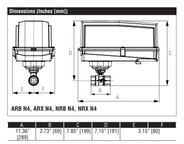
Modulating, Non-Spring Return, 24 V, for 2 to 10 VDC or 4 to 20 mA
