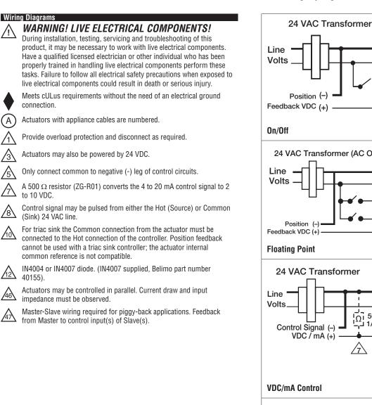
46 /47 24 VAC Transformer (AC Only) Ω Blk (1) Common Red (2) + Hot Wht (3) Y, Input Pnk (4) Y Input Org (5) U Output /47 46 Blk (1) Common + Hot Red (2) וֹם 500Ω i 1/4 watt Wht (3) Y Input  $\sqrt{7}$ Pnk (4) Y<sub>,</sub> Input Org (5) U Output 24 VAC Transformer (AC only) A 46 /47 Blk (1) Common Red (2) + Hot Wht (3) Y, Input Y, Input Pnk (4) Position (-) Feedback VDC (+) Org (5) U Output
