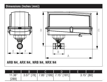
LF24-SR US, Valve Actuator Modulating, Spring Return, 24 VAC for 2 to 10 VDC or 4 to 20 mA Control Signal
