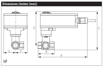
LF24-SR-S US, Valve Actuator Modulating, Spring Return, 24 VAC for 2 to 10 VDC or 4 to 20 mA Control Signal
