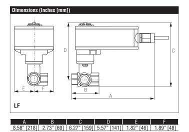
LF24-MFT-S US, Valve Actuator Modulating, Spring Return, 24 V, Multi-Function Technology®
