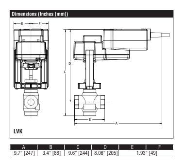
LF24-SR US, Valve Actuator Modulating, Spring Return, 24 VAC for 2 to 10 VDC or 4 to 20 mA Control Signal
