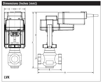
LF24-SR US, Valve Actuator Modulating, Spring Return, 24 VAC for 2 to 10 VDC or 4 to 20 mA Control Signal
