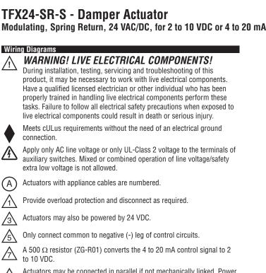
Actuators may be connected in parallel if not mechanically linked. Power /1\ consumption and input impedance must be observed.
