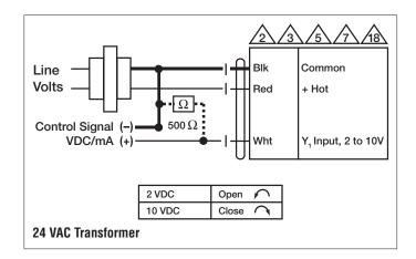
Modulating, Non-Spring Return, 24 V, 2 VDC Open 10 VDC Close or 4 to 20 mA
