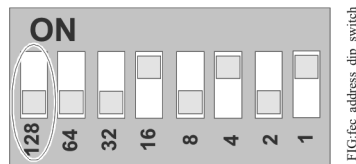
Figure 9: Device Address DIP Switch Block Set to Address 21
