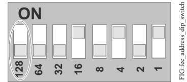
Figure 9: Device Address DIP Switch Block Set to Address 21
