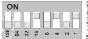
Figure 10: Device Address DIP Switch Block Set to Address 21
