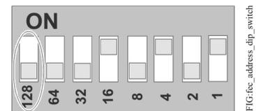
**Note:** Switch 128 is used to enable or disable a controller for wireless operation.
