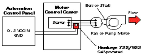
■ These sensors need no external power supply. Adjustable span gives you best resolution.
