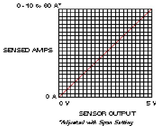
■ H-722 & H-922 require 1 A & 3 A monitored current for turn-on, respectively. Wrap conductor if lower turn on is required. 2% accuracy is achieved when monitored current exceeds 10% of scale selected.
