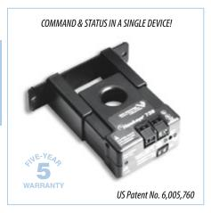
The Hawkeye 735 Series is the ideal solution for the automation installer. These units combine a current switch and relay into a single package, reducing the space required for total control of fans and pumps. The integral current switch and relay operate independently of one another. The 735-759 products facilitate the functions of start/stop and status with one device instead of two.
