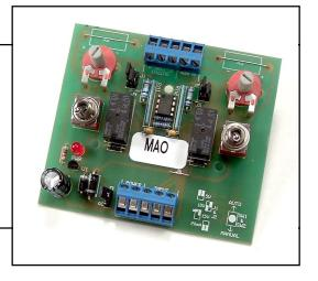
output and vary the analog signal independently. Each output can have a different span and be analog current or voltage. When a switch is in manual position, an alarm output contact is made or broken (optional) to indicate override is in effect.
