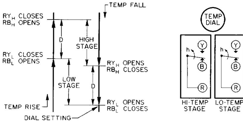
**Fig. 3: Switching action of the two-stage control is illustrated above. RB<sub>H</sub>, RY<sub>H</sub> indicates HI-TEMP stage; RBL, RYL indicates LO-TEMP stage. "D" represents the differential between stages.**
