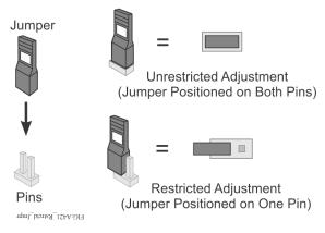
Control adjustment is now restricted to changing only the OFF value, which shifts the On and OFF control band within the restricted adjustment range defined by HtS and LtS (Figure 9).
