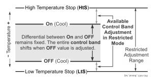
Setting the control to Restricted Adjustment mode
