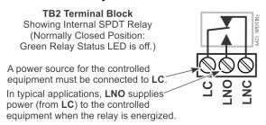
You can also provide an independent power source for the A421 Control on the TB1 terminals and then wire the TB2 relay terminals to a separate power source to switch and power the controlled equipment circuit.
