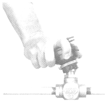
Figure 3: Tilt the actuator over the bonnet.
