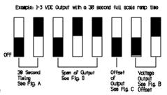
time to insure that the analog output is at maximum. The input signal will NOT "wrap around" or start over if the upper range limit is exceeded. Then set the Span trimmer potentiometer to the desired maximum output signal (measured between terminals PWR (-) and SIG.
