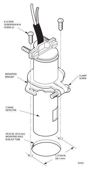
Fig. 8. Mounting C7044A Detector on blast tube.
