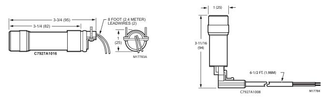
Fig. 4. Installation dimensions of C7927A1016 (U.S.A. version) and C7927A1008 (European version) in in. (mm).
