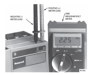
Fig. 11. Measuring flame signal voltage of 7800 SERIES controls.
