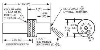
$\Delta$  DIN APPROVED C7035A1064 HAS 1-11 BSP.P1 INTERNAL MOUNTING THREADS.  $\Delta$  DIN APPROVED C7035A1064 HAS 1/2-14 BSP-F INTERNAL MOUNTING THREADS.
