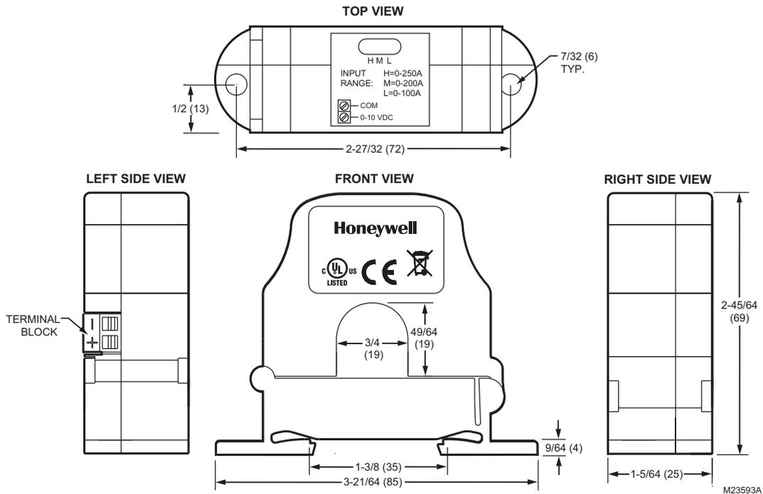
Fig. 2. CTP current sensor dimensions in inches (mm)
