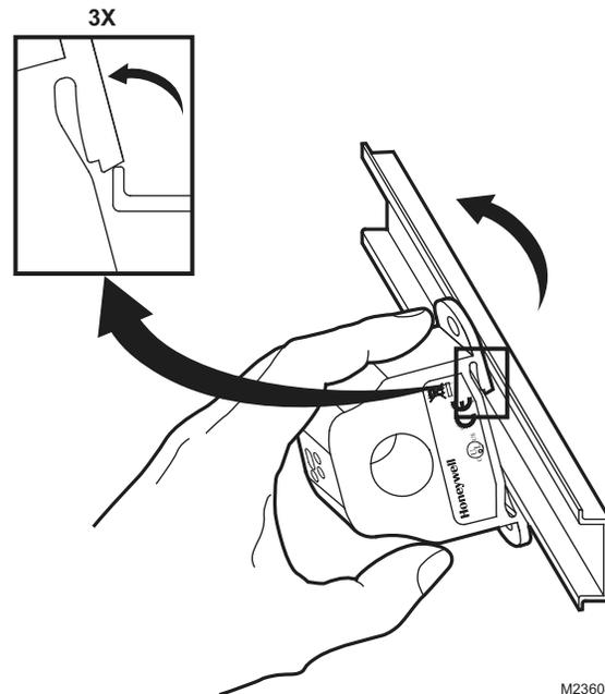
**Fig. 4. Sensor removed from DIN rail**
