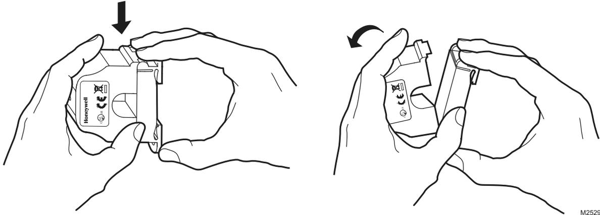
Fig. 5. Opening sensor by hand
