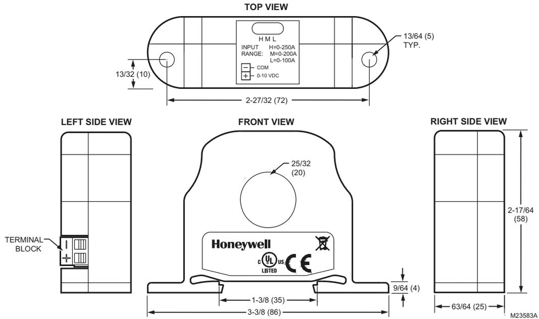
Fig. 1. CTS current sensor dimensions in inches (mm)
