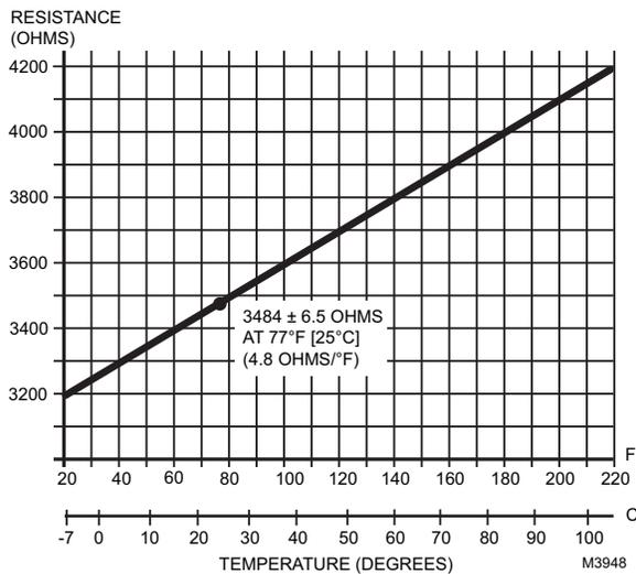
**Fig. 2. Variation of C7170 Sensor resistance as compared to temperature.**
