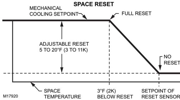
Fig. 7. Space reset algorithm.
