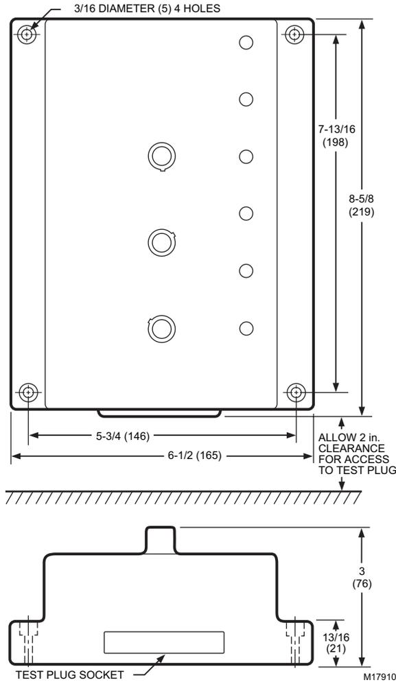
**Fig. 1. W7100 Discharge Air or Water Controller mounting dimensions in in. (mm).**
