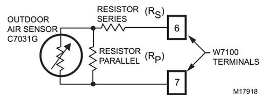
Fig. 10. Reset modification schematic wiring diagram.
