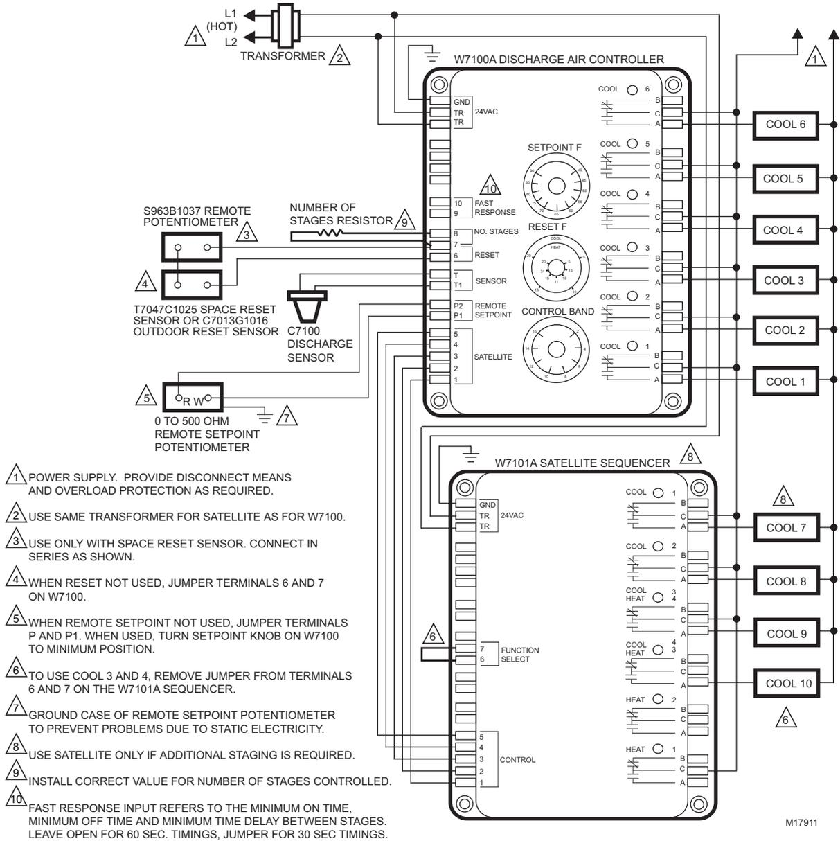
**Fig. 4. Connections for W7100G 10-stage cooling, with W7101 Satellite Sequencer, discharge sensor, reset sensor(s) and remote setpoint potentiometer.**
