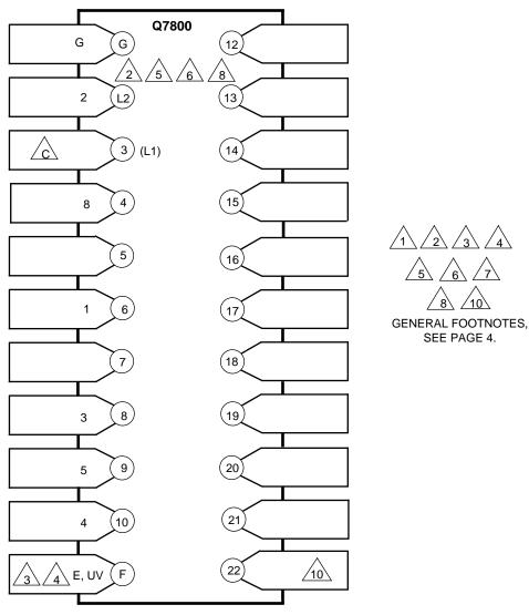
THESE DEVICES TYPES WOULD LOCKOUT ON A FLAME FAILURE. TO MAINTAIN THIS FUNCTION, JUMPER 2 OF THE RM7890 DEVICE MUST BE CLIPPED. REFER TO SPECIFICATION, FORM 65-0126.
