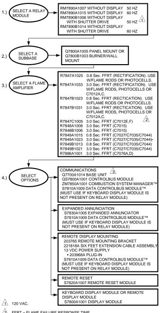
2 FFRT = FLAME FAILURE RESPONSE TIME.
