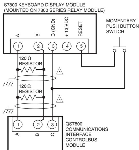
⚠ THREE WIRE SHIELDED CABLE MAY BE REQUIRED. TWO 120 OHM TERMINATING RESISTORS ARE REQUIRED FOR CONNECTIONS OVER 100 FEET [30 METERS]. CABLE SHIELD MUST BE TERMINATED TO EARTH GROUND AT BOTH ENDS. IF SHIELDED CABLE IS NOT USED, TWISTED PAIR WIRE MUST BE USED.
