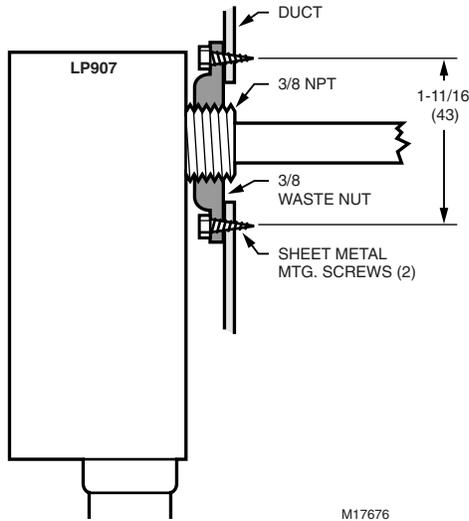
Fig. 2. Mounting on standard sheet metal duct.
