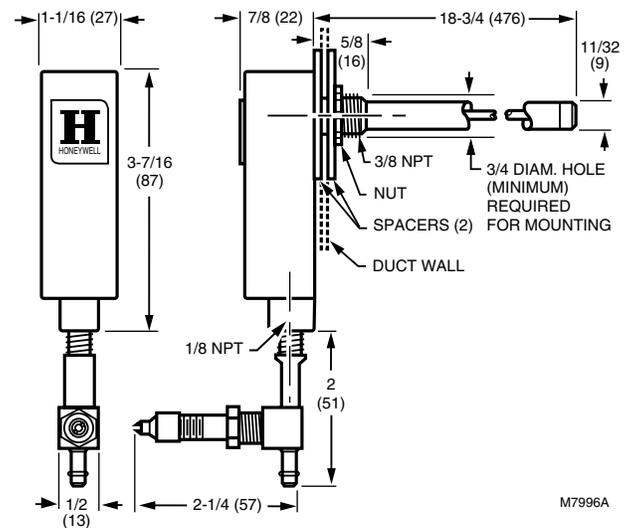
Fig. 1. Dimensions of LP907A in in. (mm).
