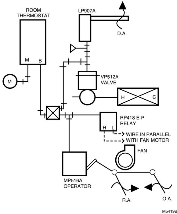
Fig. 5. Typical operation.
