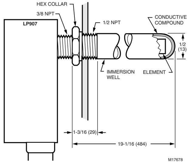
Fig. 4. Mounting in boiler wall with immersion well.
