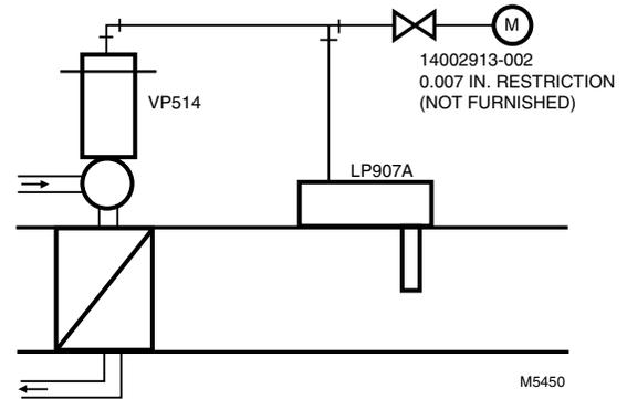
Fig. 7. Typical operation of duct mounted LP907A.
