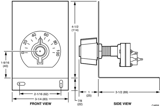
Fig. 2. SP970B and D dimensions in in. (mm).
