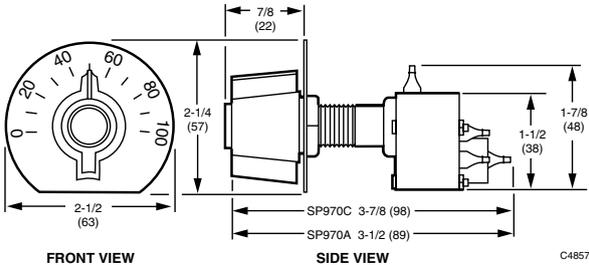
Fig. 1. SP970A and C dimensions in in. (mm).
