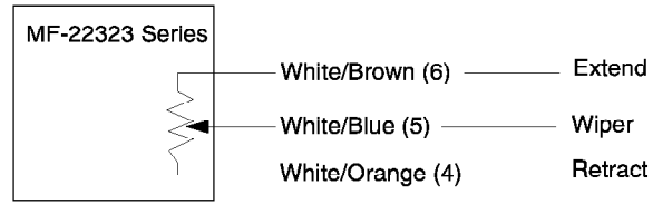
Figure-5 MF-22323 Feedback Wire Designations.
