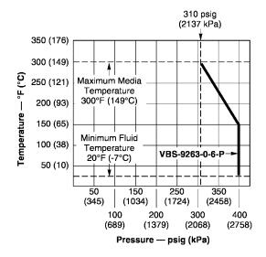
Figure-2 Temperature and Pressure Ratings for VBS-9263 Series Valve Bodies.
