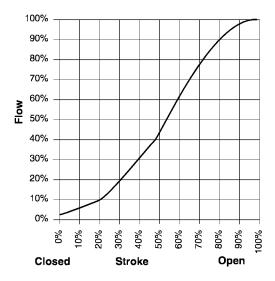
Figure-1 Typical Modified Equal Percentage Flow Characteristics.
