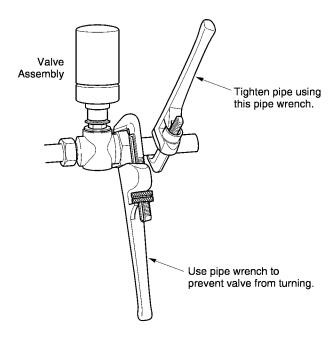
Figure-4 Installation of Screwed End Valves.
