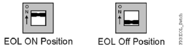
Figure 14: End-of-Line switch positions
