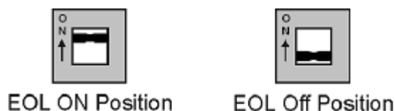
Figure 10: End-of-Line switch positions
