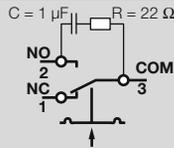
In the case of high humidity or aggressive gas components ( $\text{H}_2\text{S}$ ), we recommend using a pressure switch with gold contact due to its higher resistance to corrosion. Closed-circuit current monitoring is recommended under difficult operating conditions.
