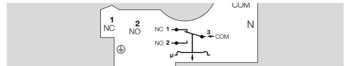
Contacts 3 and 2 close when subject to increasing negative pressure. Contacts 1 and 3 close when subject to falling negative pressure.
