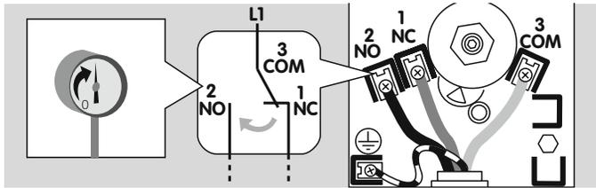
Contacts 3 and 2 close when subject to increasing pressure. Contacts 1 and 3 close when subject to falling pressure.
