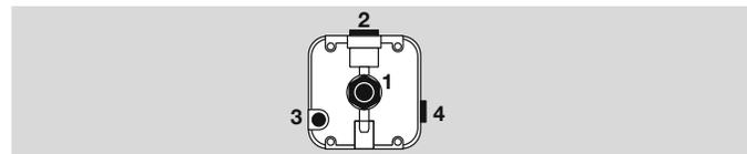
Ports 3 and 4 are connected to the micro switch chamber. The port that is best protected against soiling (dust/humidity) is to be left open for ventilation (positive pressure measurement) to the atmosphere. If dust exposure in the environment is high, a filter pad, see page 20 (Restrictor orifice), or a filter are to be used in the open port.
