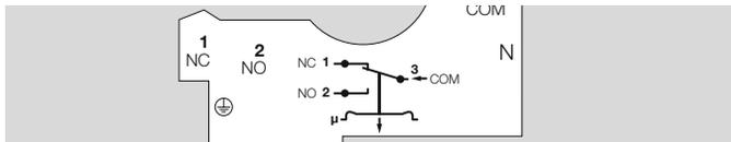
In the positive adjusting range, remove the template and wire the unit as shown in the engraved connection diagram.
