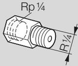
In the case of high pressure fluctuations, we recommend using a restrictor orifice (contains non-ferrous metals):
