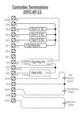
BI-O:: Motion Detector PIR (optional) BI-1:: Door/Window Sensor (optional) BI-2:: Main Door Sensor (optional)
